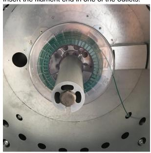
TIP: If insert more than one spool inside the chamber place it at opposite direction as previous spool to avoid filament tangling.
