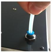
To remove tube, press blue ring and take the tube out:
