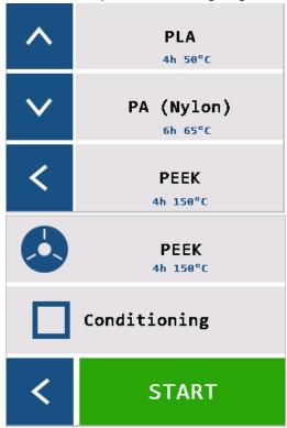
Once material is chosen there is an overview of the drying settings and possible to disable/enable conditioning (if enabled then after drying it will keep 40C in the chamber to keep it dry longer). When pressed Start button warming up will automatically started.
